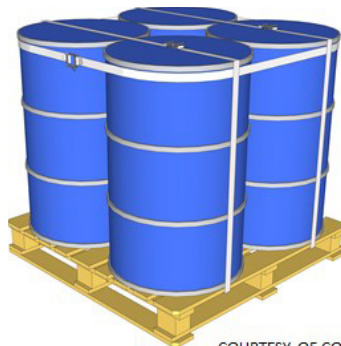
Figure 5.5 Drums secured to pallet with strapping
