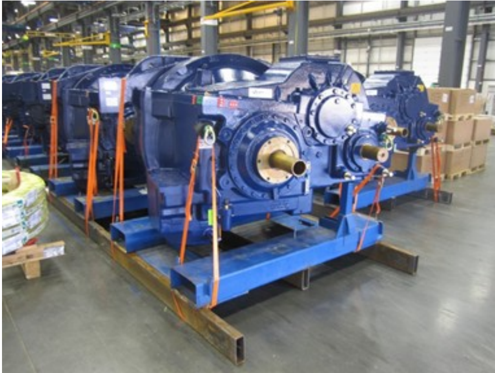
Figure 6.8.2 - 1 - Gearboxes mounted on sled Method 6.8.2 - Gearboxes mounted on sleds in 20-ft ISO containers
